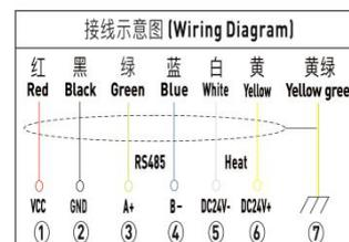
UART output: it is recommended to use RVVP/0.5mm<sup>2</sup>/copper core/high and low temperature resistant shielding cable, maximum communication distance is 200m.
